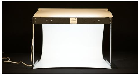
Basically, the box is made to have white walls or a white backdrop, which allows the light to just bounce all around what you want to take a picture of, so that you can effectively eliminate all shadows.
